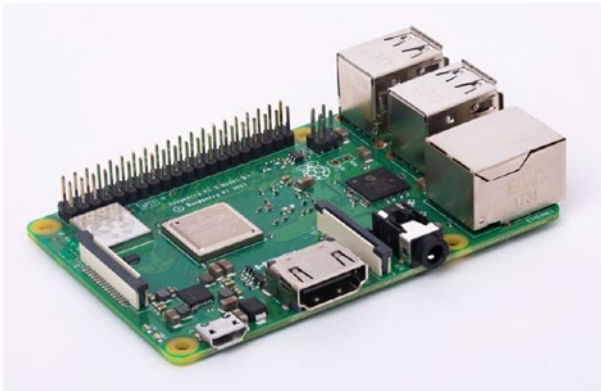
Figure 1-1. Raspberry Pi 3 B+ board
