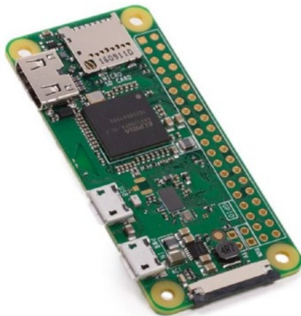
Figure 1-2. Raspberry Pi Zero Wireless board
