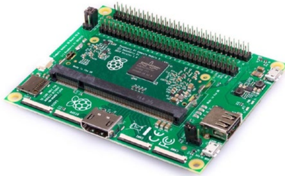
Figure 1-3. Raspberry Pi Compute Module v3
